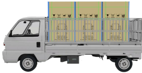
Figure 9 Securely fasten the assembly to the lorry
